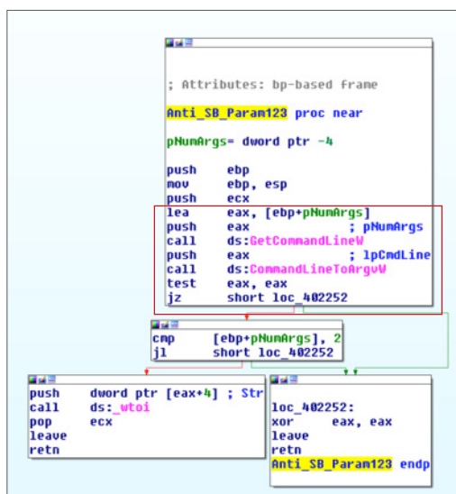
Figure 18: In this example, the command-line parameter “123” is passed by the infection vector, a JavaScript file. Then, the command-line parameter is read by the Windows API GetCommandLine and CommandLineToArgvW . (Hash: 0fed77b29961c0207bb4b7b033ca3fd4)
